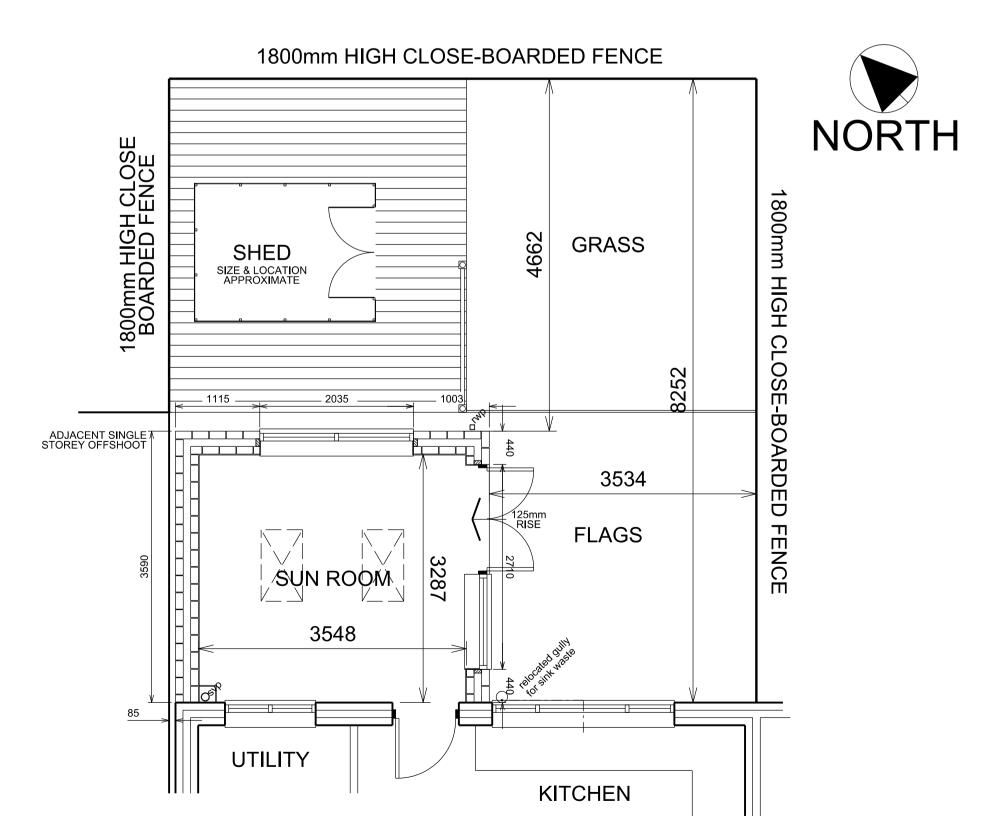
PROPOSED SITE / PART FLOOR PLAN (1:50)
